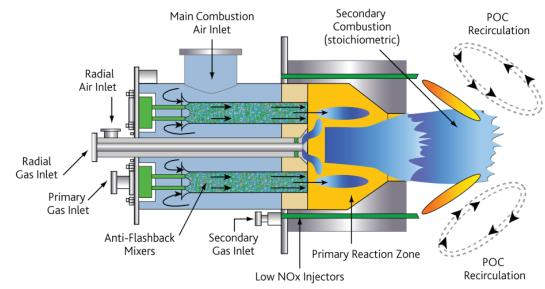
Figure 2. The Magna-Flame LE is a staged fuel burner design with lean burn primary combustion zone. The balance of the fuel is injected downstream.
