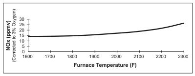
Figure 3. NOx Emissions vs. Furnace Temperature.
