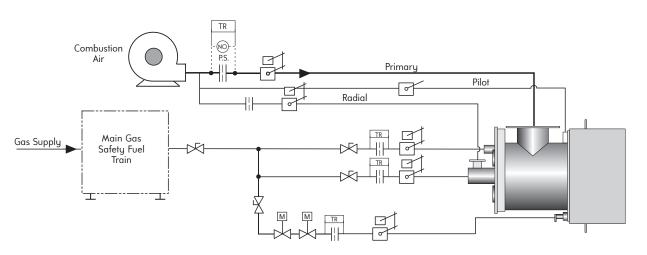
Figure 2. Typical Piping Schematic for LE Cold Air System.
